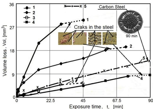
Fig.7. Volumetric losses and degradation of the layers deposited by thermal spraying exposed to vibratory cavitation
