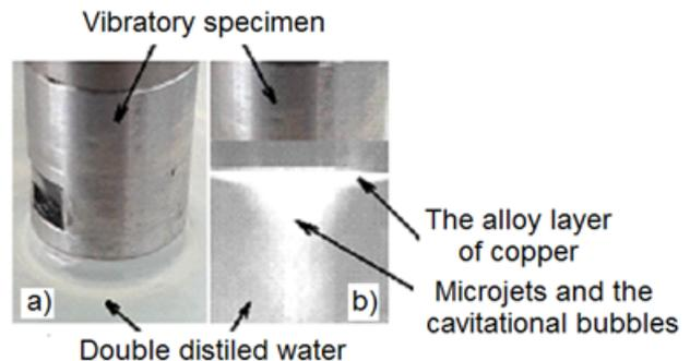
Fig.6. Vibratory specimen (recordings made in TPU Cavitation Laboratory) a) static specimen; b)vibrating specimen
