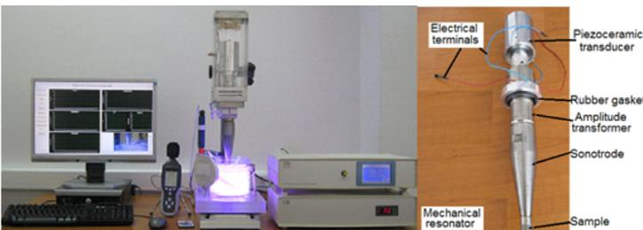
Fig.4 Standard vibratory device (Timisoara Polytechnic University, Cavitation Laboratory)
