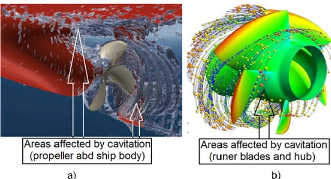
Fig.5 Images of flow with cavitation [7, 8]
