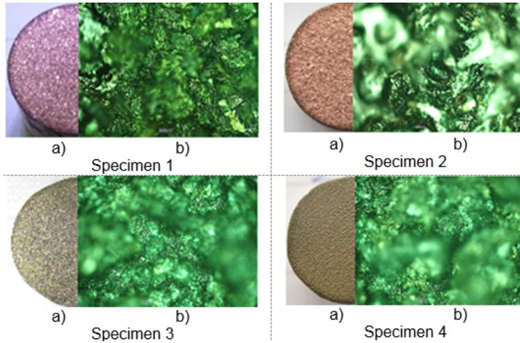
Fig.2 Surfaces subjected to thermal spraying
